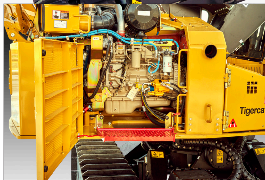
Easy access to daily engine service points.
