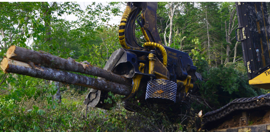
Excellent multi-stemming for enhanced productivity in small diameter timber.
