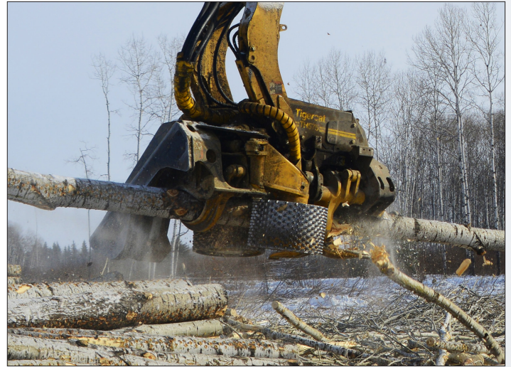
Maximum feed force in three-wheel drive for large limbs, big wood.
