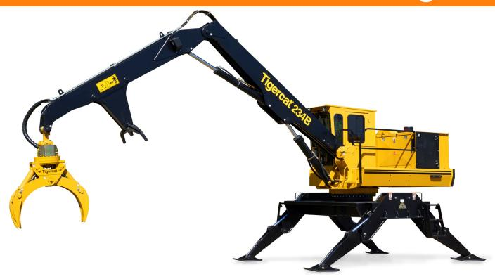
The 234B series loaders are an excellent choice on the deck or in the mill yard. The 234B and T234B are designed and built for high production logging operations and high duty cycle delimbing.
