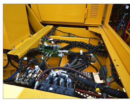
All valves are located underneath the walk-up platform for clear and easy access with neat hydraulic and electrical routings.
