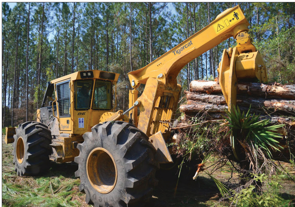
High capacity dual cylinder grapples and high visibility arch.
