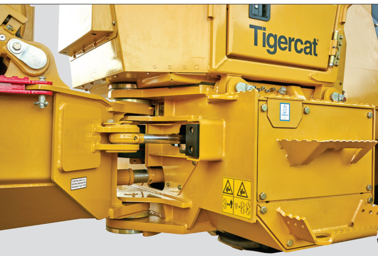
Strong centre section with large pins and tapered roller bearings.
