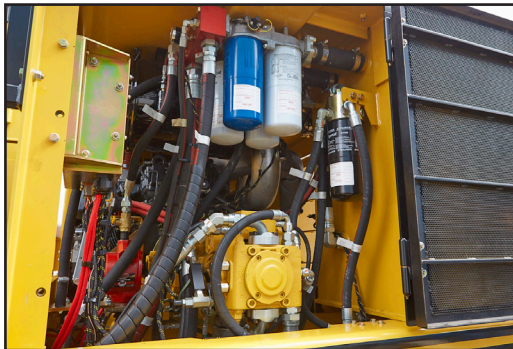
Swing-out access to the hydraulic pumps and filters
