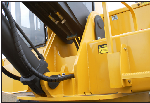
Large pins and thick steel plate at boom pivots for long, trouble-free service life
