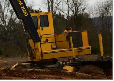
Optional bunk and stakes for additional carrying capacity. Combined with a trailer, the AC16 has the potential to quickly move large volumes of timber around the yard.
