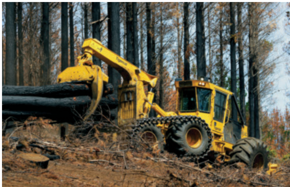
A 615C skidder salvaging burnt timber in Chile.
