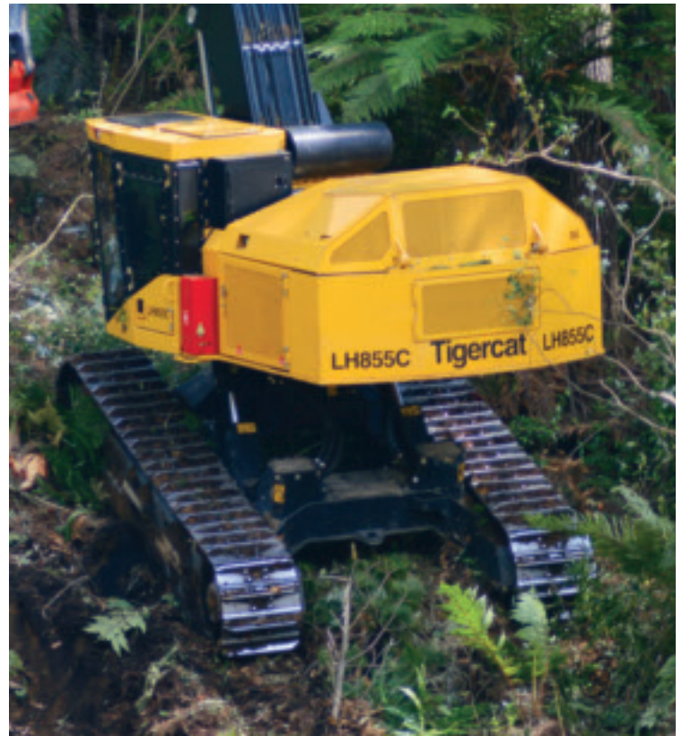
Drives at the back to get the most pin and bushing life.
