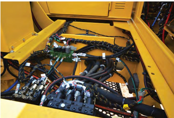
All valves are located underneath the walk-up platform for clear and easy access with neat hydraulic and electrical routings.
