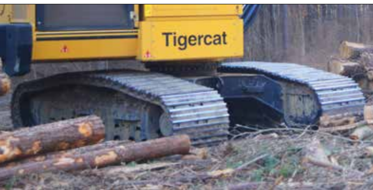
Tigercat-built full forest duty undercarriage with powerful tractive effort for excellent mobility in tough terrain. Long track frames and wide stance for comfort and stability.
