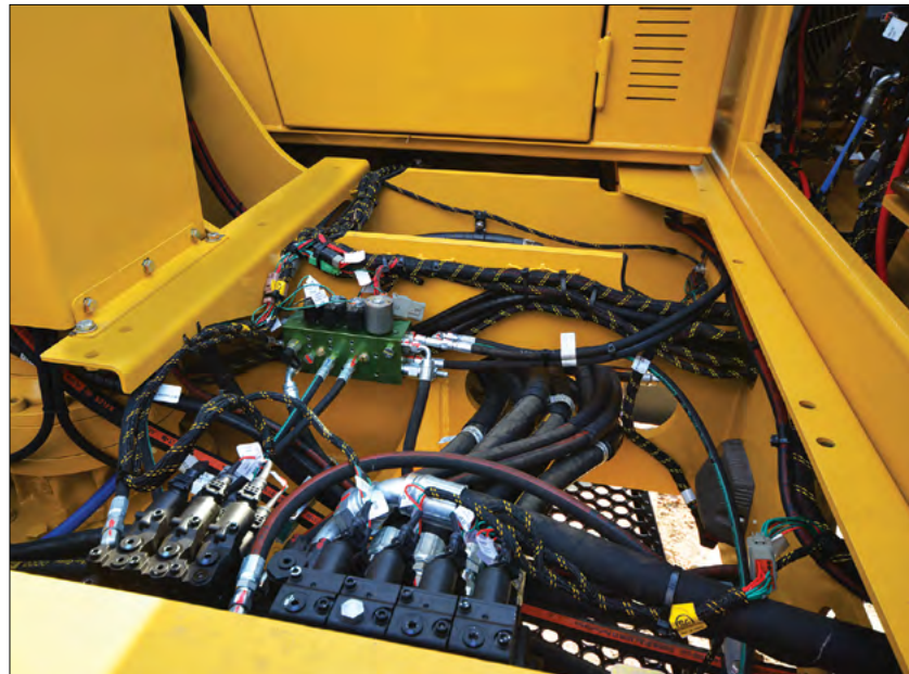
All valves are located underneath the walk-up platform for clear and easy access with neat hydraulic and electrical routings.
