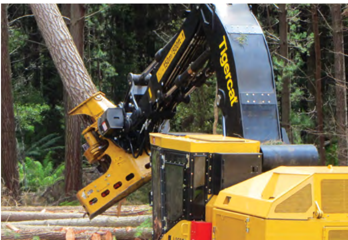
High torque 340° wrist for increased versatility and reduced machine travel.
