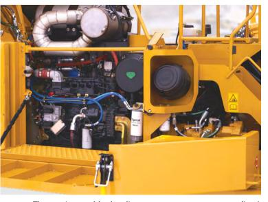
The engine and hydraulic pumps are compartmentalized and easily accessed. Easy access to daily service points.
