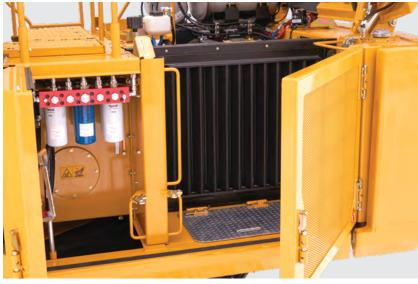
Swing-out doors access filters and cooling system components for quick daily service.
