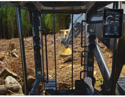
Excellent cab ergonomics and clear visibility to the track tips through the full length front window with narrow side posts. SkyVIEW camera system for expansive upward field of vision.
