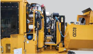
Access to both sides of the engine and aftertreatment components. Unprecedented in the zero tail-swing feller buncher class.
