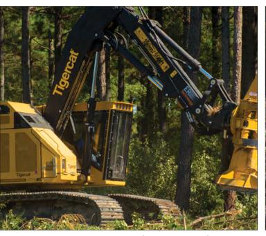
Tight tuck boom geometry for excellent performance in thinning applications, combined with clear sightlines to the right side through the extended length window.
