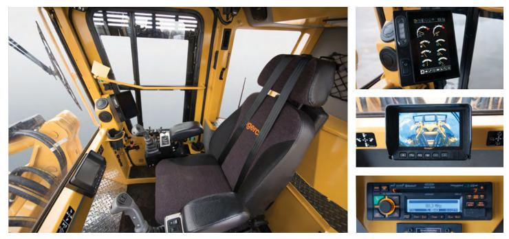
Well appointed operator's station, featuring large LCD touch screen, front/rear cameras, AM/FM CD stereo with Bluetooth® Audio and hands free calling.
