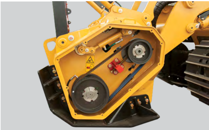
Easy access to service timing belt.
