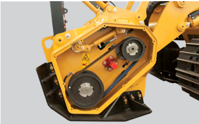
Easy access to service timing belt.
