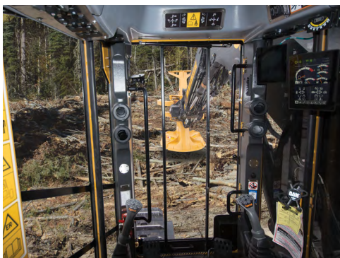
Enhanced cab with expanded sight lines and an upgraded interior finish. SkyVIEW and RearVIEW camera system.
