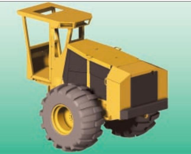
A 3-D model of a 720 rear chassis created with SolidWorks.
