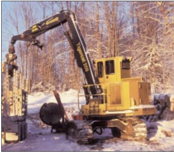
The T250 equipped with a circle saw slasher. "No one else has a circle saw on a track loader," explains Mitchell.
