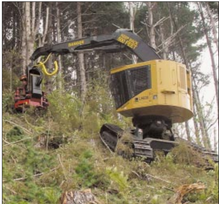
The LH830 harvester felling radiata pine on a steep grade in New Zealand's Spirits Bay.
