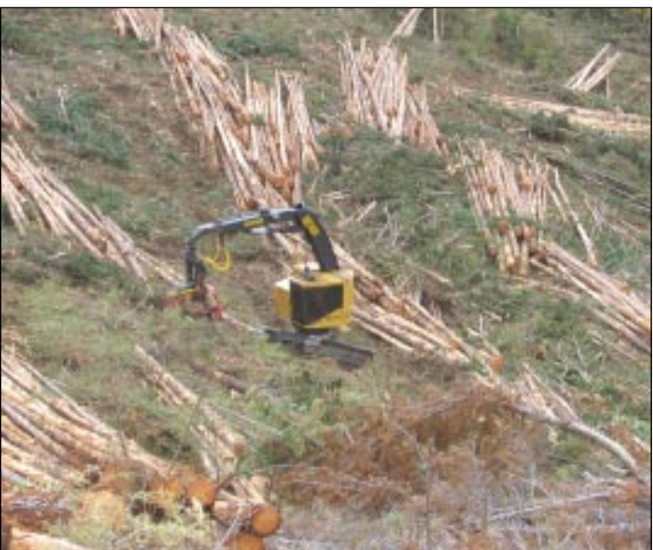
The LH830 bunches the processed stems for the swing yarder.
