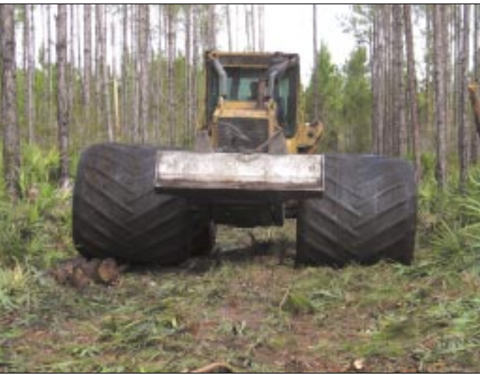
Even at 15 ft. - 10 in. wide the machine can operate effectively in the thinning corridors.
