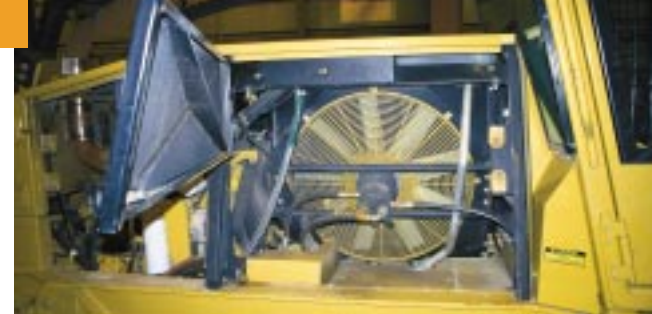
Cross-flow cooling system on a nearly assembled Tigercat skidder.
