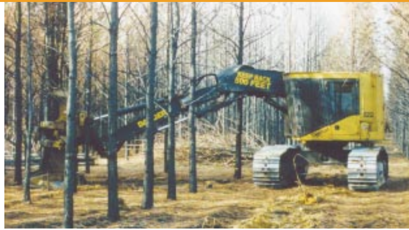
The Tigercat 822 with ER boom system quickly reaches out to harvest a tree.
