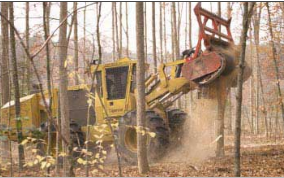
The M760 effectively mulches standing trees.
