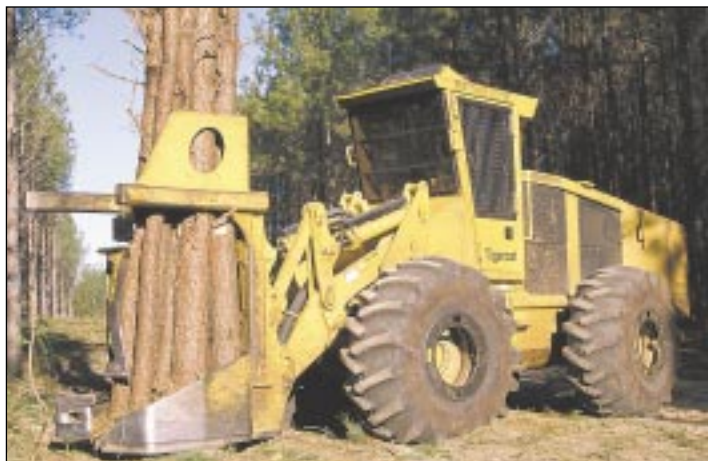
The 1800 series bunching shear. Kurelek solved the stem alignment problem with the innovative 2-arm configuration.
