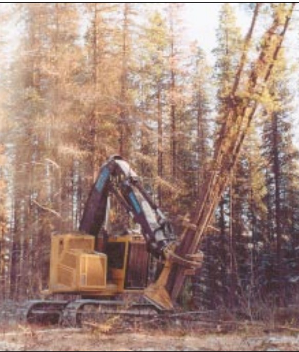
An extension to the Tigercat 822's rear end accommodates a large counterweight, which helps with the machine's ability to pick up wood at full reach.
