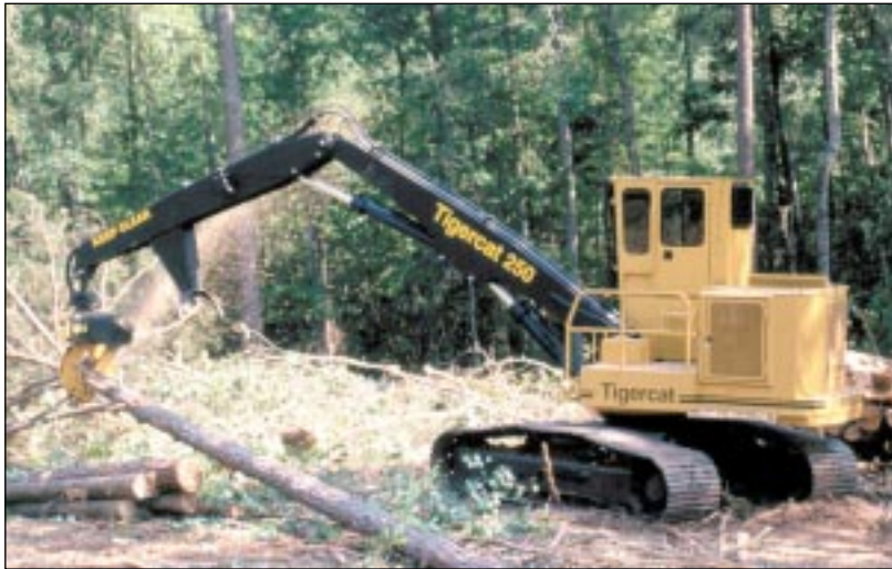
A T250 loader equipped with a Hultdins grapple saw worked the deck.
