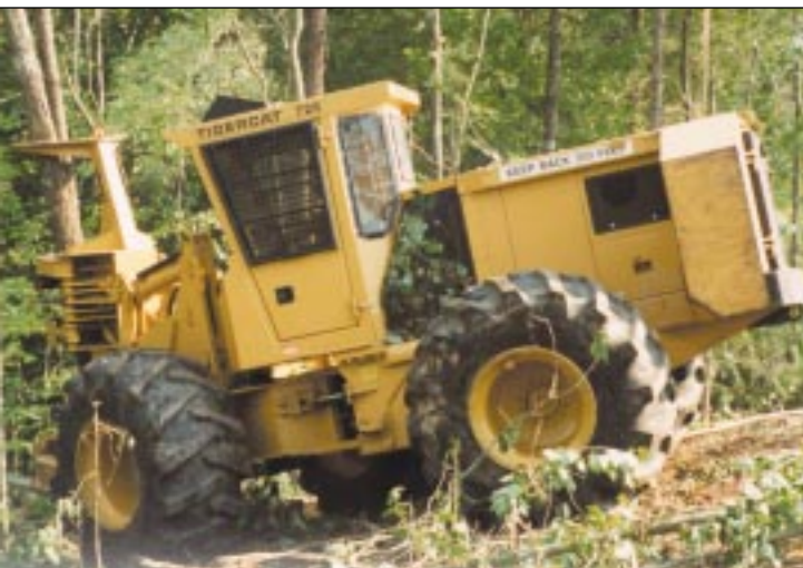
An early Tigercat 726 feller buncher. Kurelek's ideas for a better drive-to-tree buncher materialized with this machine.
