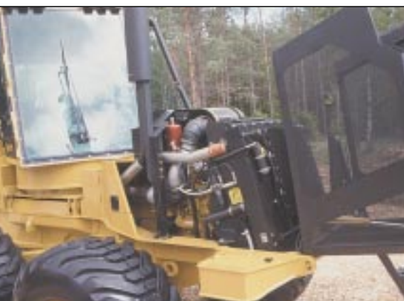
Unconventional design: rotating cab and tilt-out engine enclosure.
