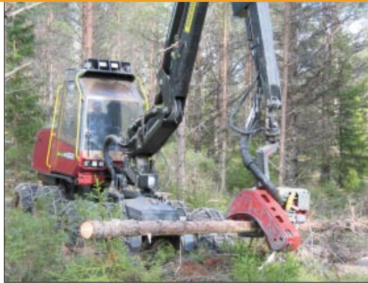
The Mowi crane tilts side-to-side to avoid standing trees.
