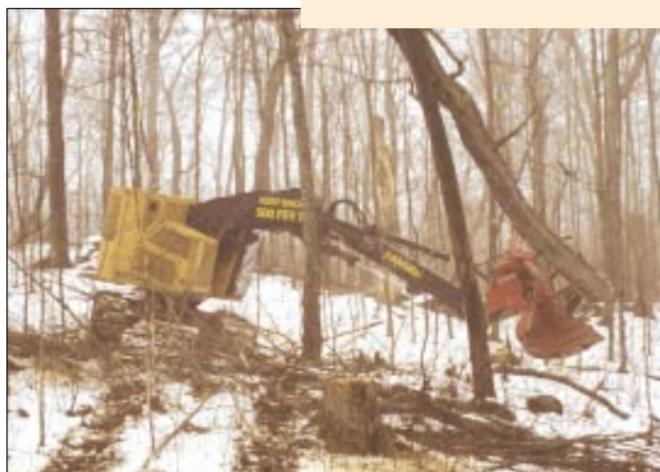
Felling large hardwoods without damaging standing trees requires a great deal of operator skill and a capable machine with ample lift capacity.
