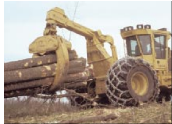
The new 630C with prototype box tongs hard at work in northern Alberta.
