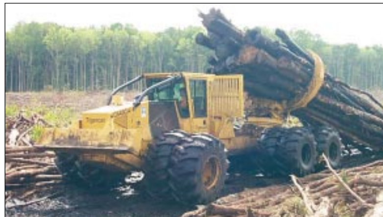
Harrison's new C640C is burning 4.5-5 (US) gal. of fuel per hour. This machine may prove to be the lowest cost, most efficient transporter available for shovel logging applications.
