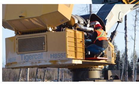
Swing-out door with service platform allowing quick and easy engine access.
