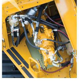
Quick and clear access to the hydraulics. Pumps and valves are separated from the main engine enclosure area.
