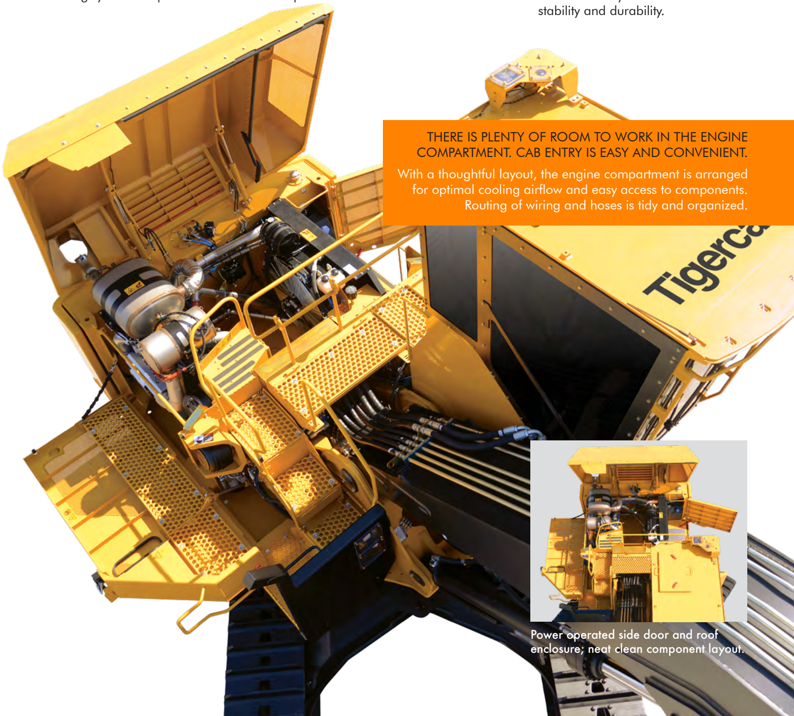
Swing-out doors for filters and cooling system components.
