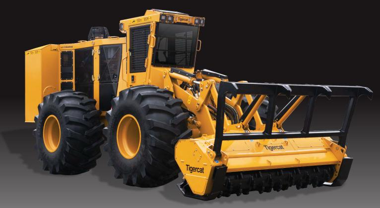
The is a durable, reliable carrier capable of powering mulching and subsoiling heads requiring up to 358 kW (480 hp). The 760B is best suited to large scale land clearing and post-harvest silviculture applications.
