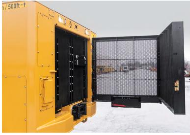
High-capacity cooling system with automatic reversing cycle.
