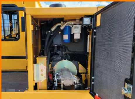
Swing-out door to access hydraulic pumps and filters.
