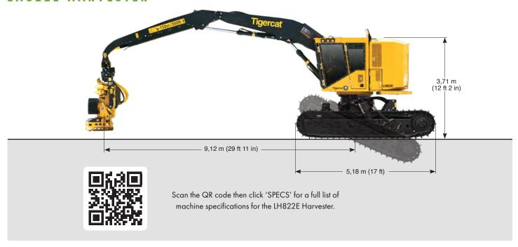
Download the Tigercat App to access the most current machine specifications for all Tigercat machine models.
