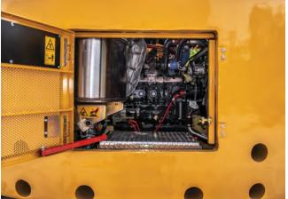
Large cast counterweight with door for additional access to the engine from the rear of the machine
