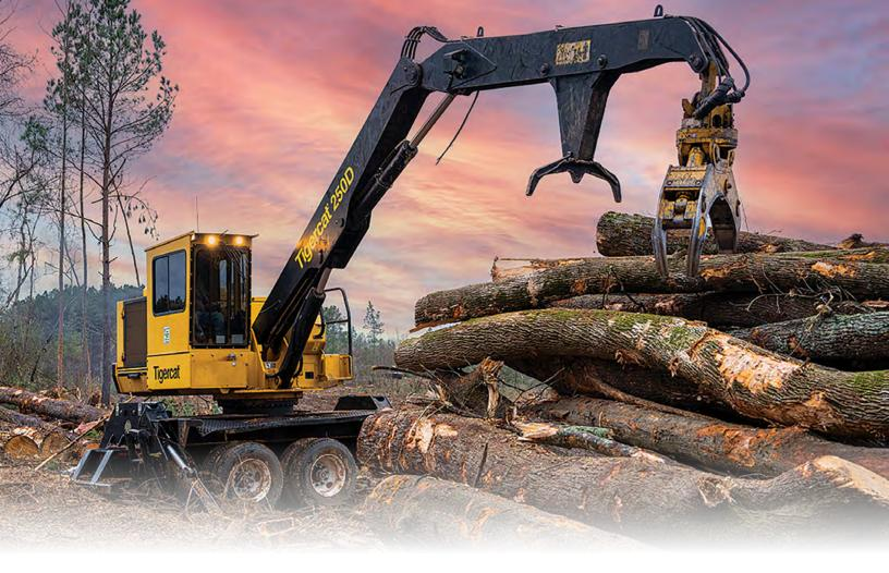
THE 250D AND T250D ARE DESIGNED AND BUILT FOR HIGH PRODUCTION LOGGING OPERATIONS, HEAVY TIMBER AND TOUGH DUTY CYCLE DELIMBING APPLICATIONS.
