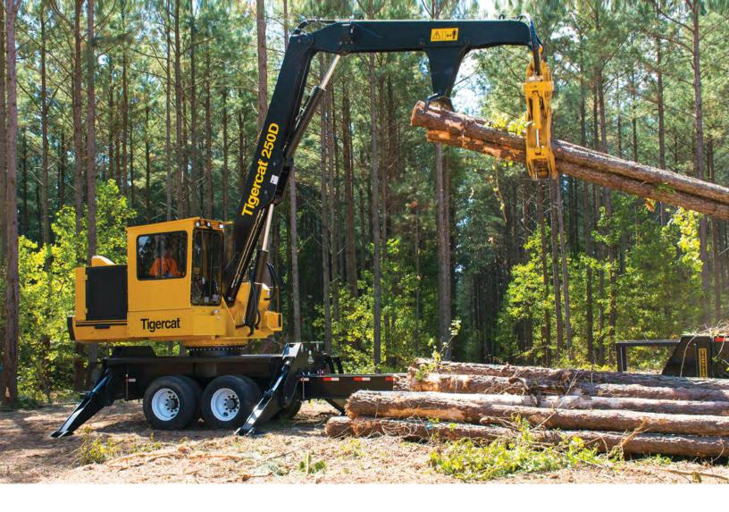
EFFICIENT HYDRAULICS WITH A CLOSED LOOP SWING SYSTEM DELIVER SIMULTANEOUS POWER TO ALL MACHINE FUNCTIONS FOR HIGH PERFORMANCE, RESPONSE AND FUEL EFFICIENCY.
