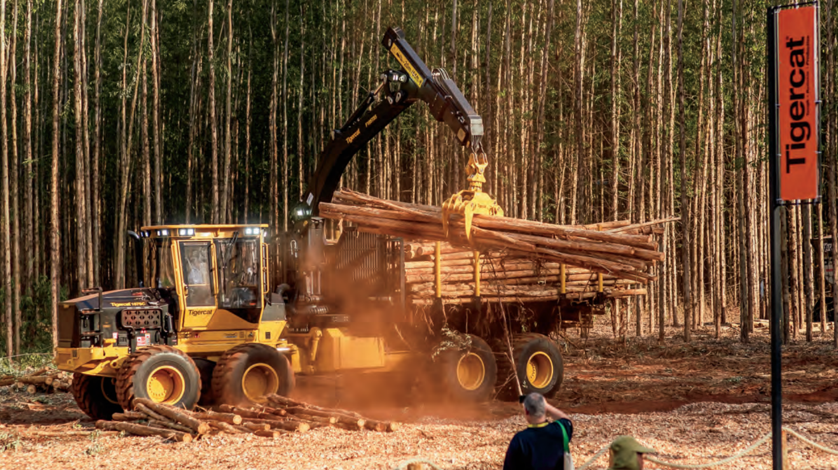
Tigercat 1075C forwarder loading seven metre lengths.
