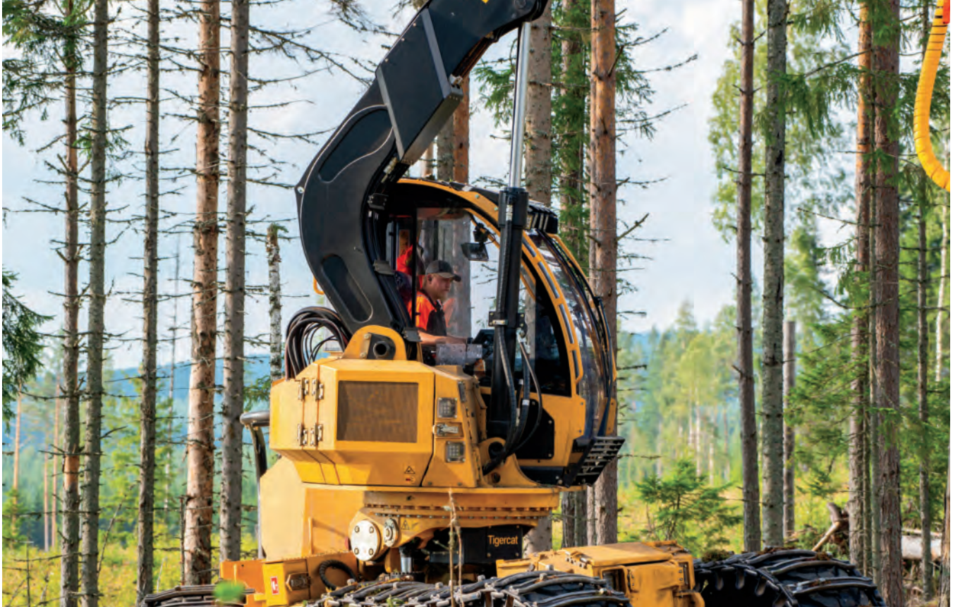
360-degree continuous cab and crane rotation is unique among harvesters.
