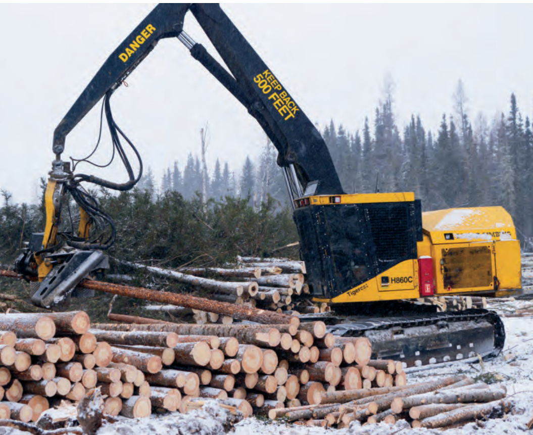
The 575 prototype mounted on a Tigercat H860C carrier about halfway through its sixteen year, 50,000 hour life.
