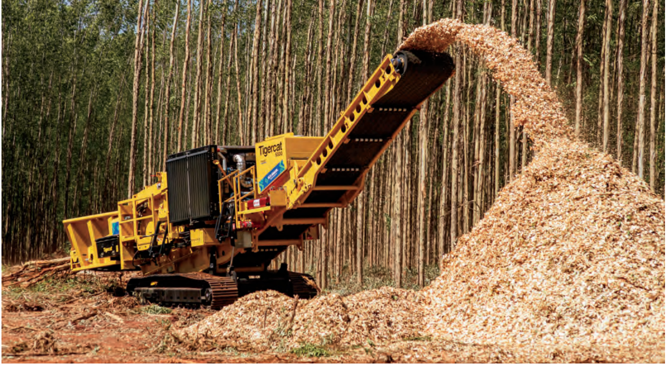
Tigercat's new 6500 material processor producing fuel chips.
