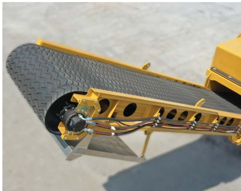
The large magnetic head pulley for tramp metal removal.
