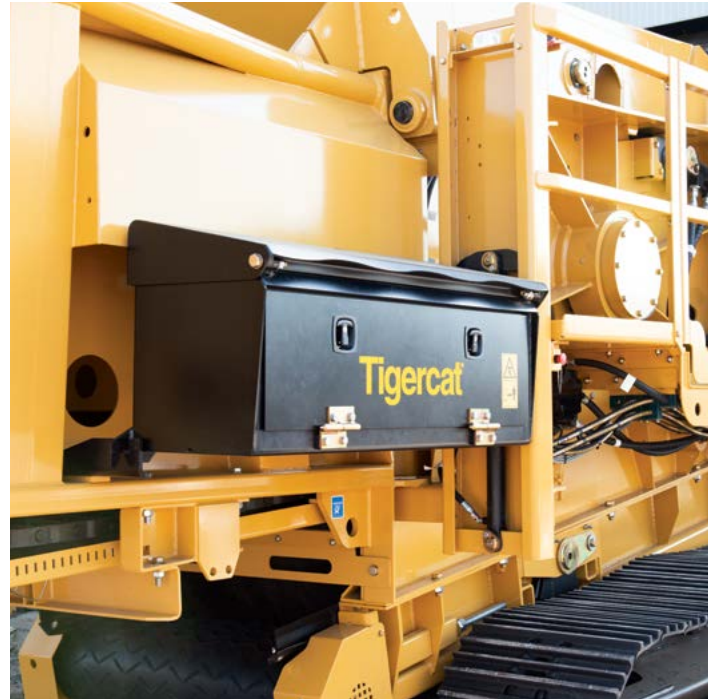
Toolbox that hydraulically raises and lowers.
