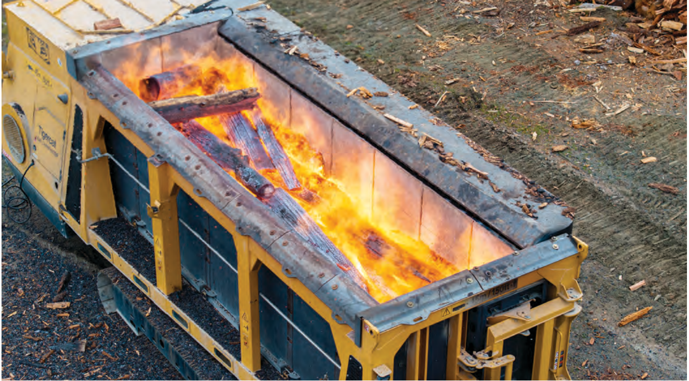
The 6040 converts 15-20 tons per hour of unprocessed woody material into a high-quality organic carbon product.
