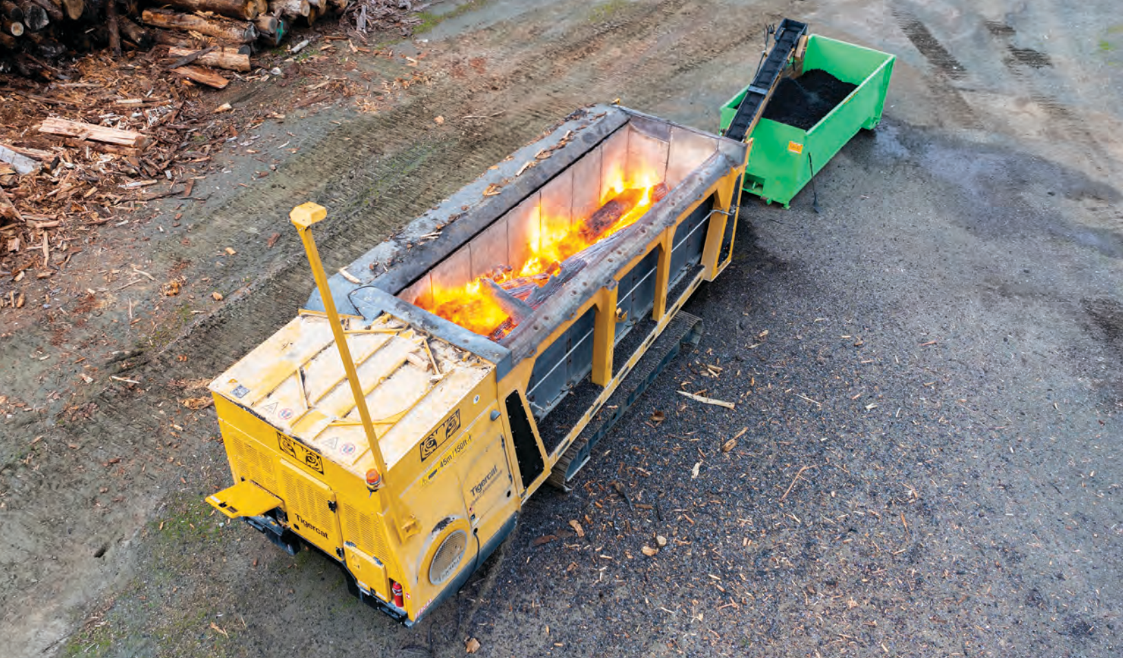
The prototype 6040 carbonizer was purchased by Falk Forestry in 2024. The machine has a number of improvements over the 6050 design.
