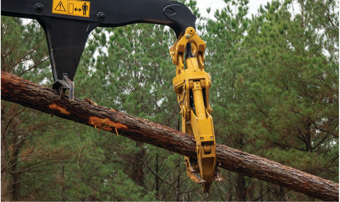
Beau appreciates Tigercat's through-tip routing, offering excellent protection for the hydraulic hoses supplying the grapple.
