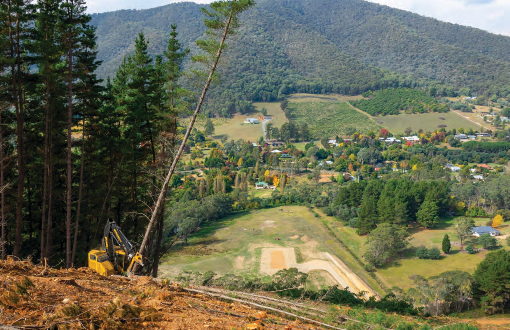
A typical yarding site in northeastern Victoria. The high rotation wrist provides precisely angled tree placement for the yarder with much less track travel required.
