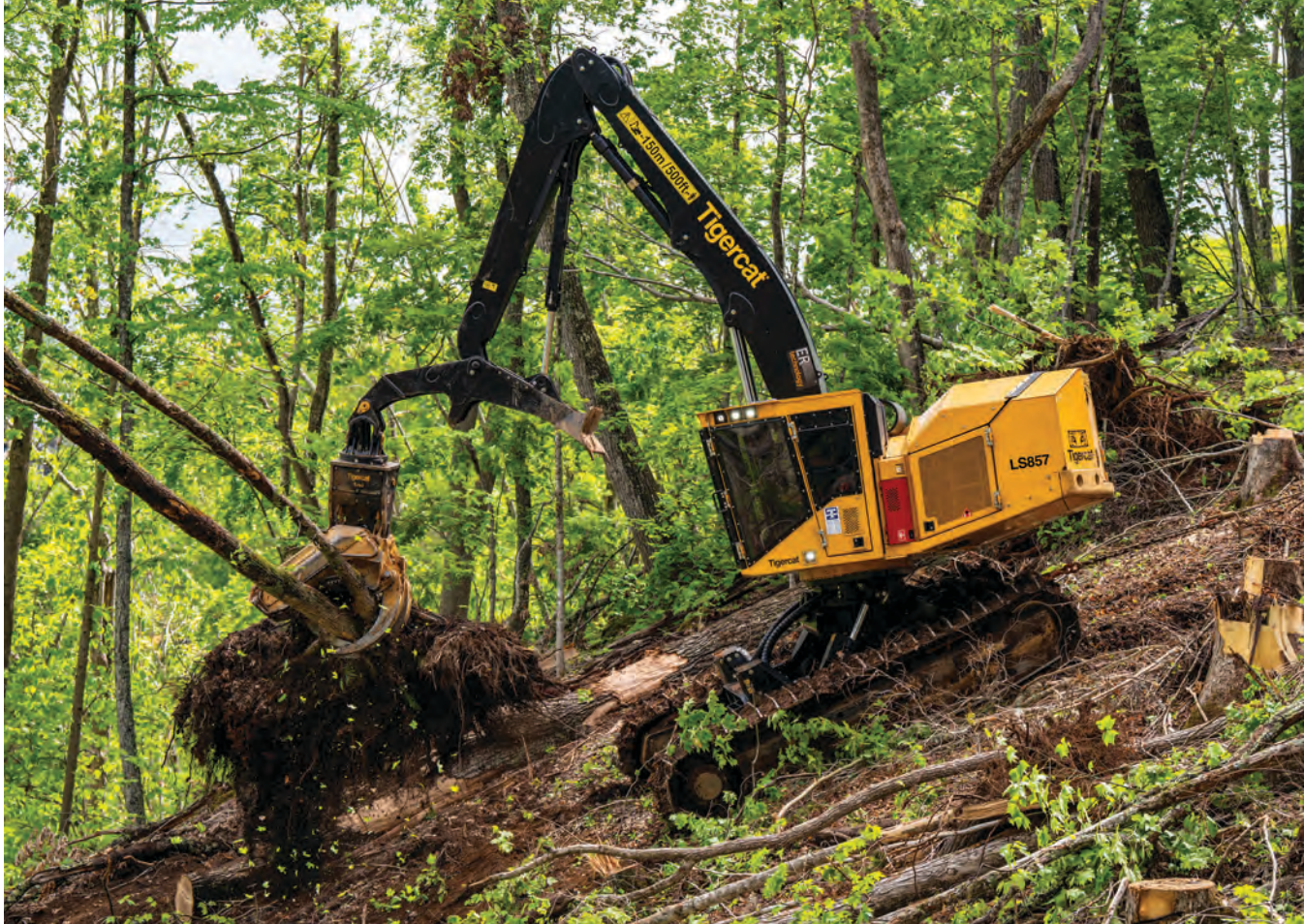
The unique profile of the LS857 provides increased leveling capability and improved cable management for winch assisted operations. The machine is paired with a 5195 directional felling saw, making the package versatile for felling, shovel logging, bunching, stacking and sorting.
