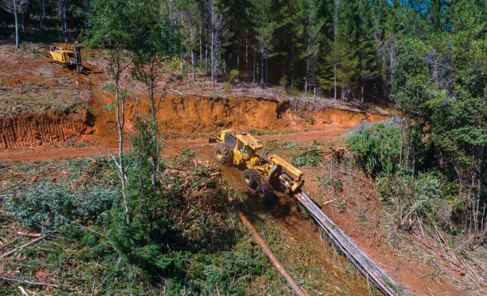
A 635G skidder working with the 120 winch assist. The 120 has full travel signal integration with Tigercat carriers.
