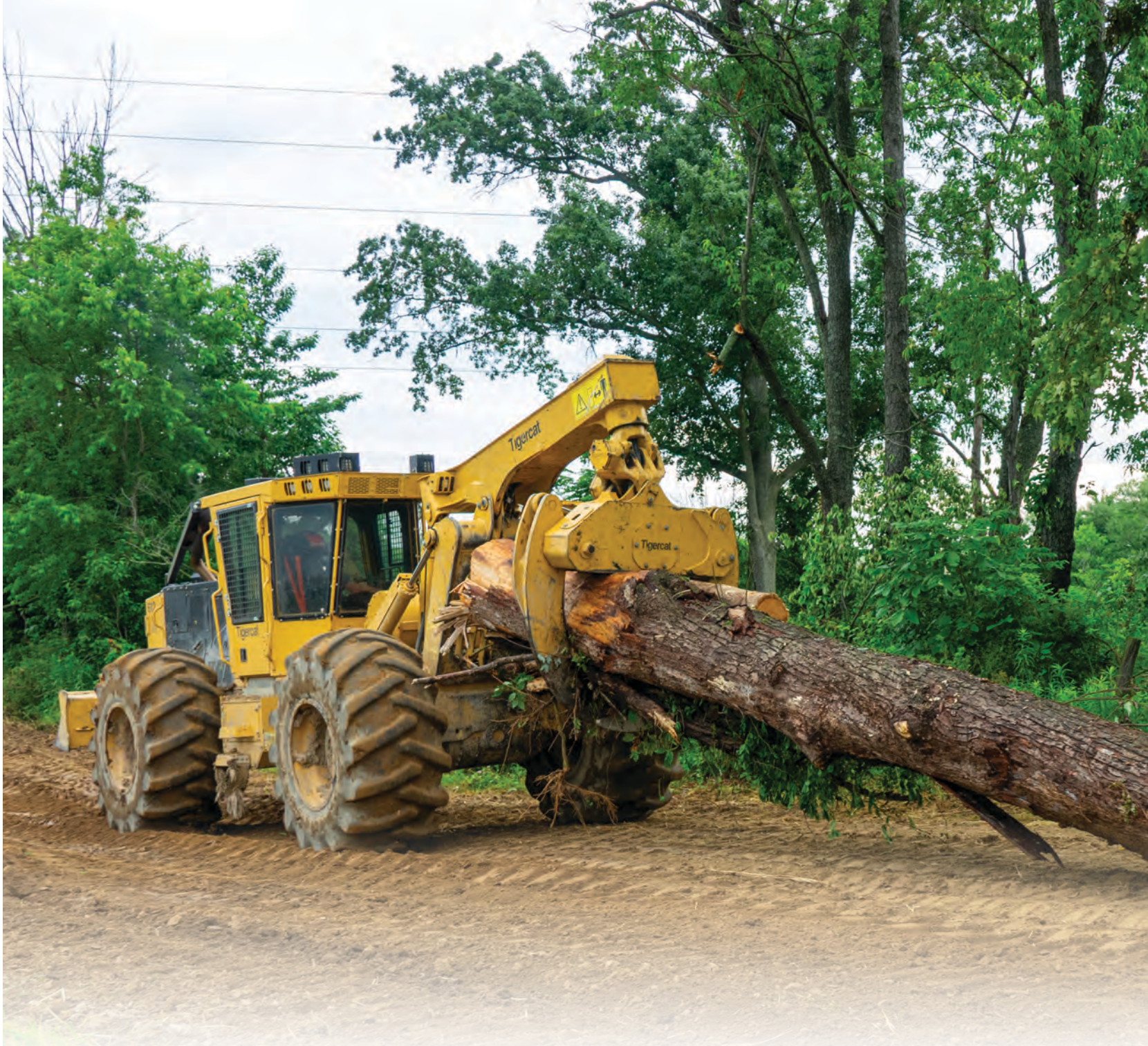
The Tigercat 612 skids large hardwood in a blowdown cleanup job in Ohio.
