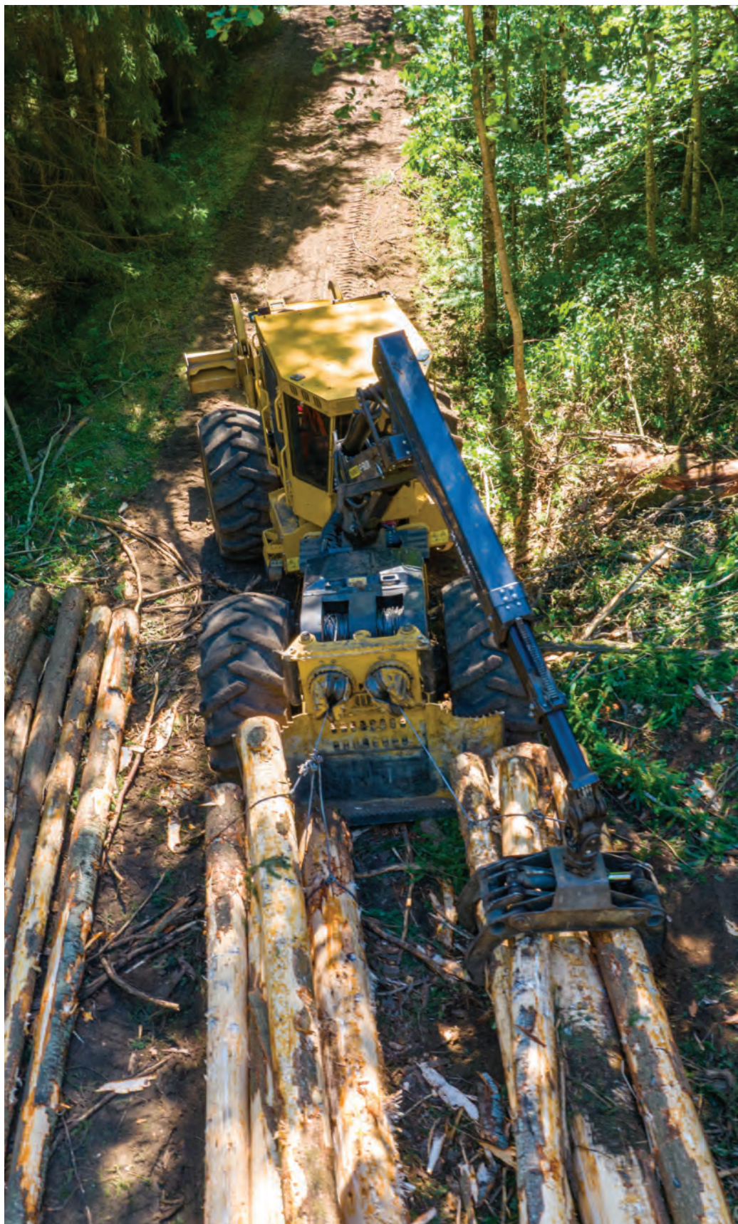
The TCi 612 skidder transports processed tree-length logs 200 metres to the public roadside.
