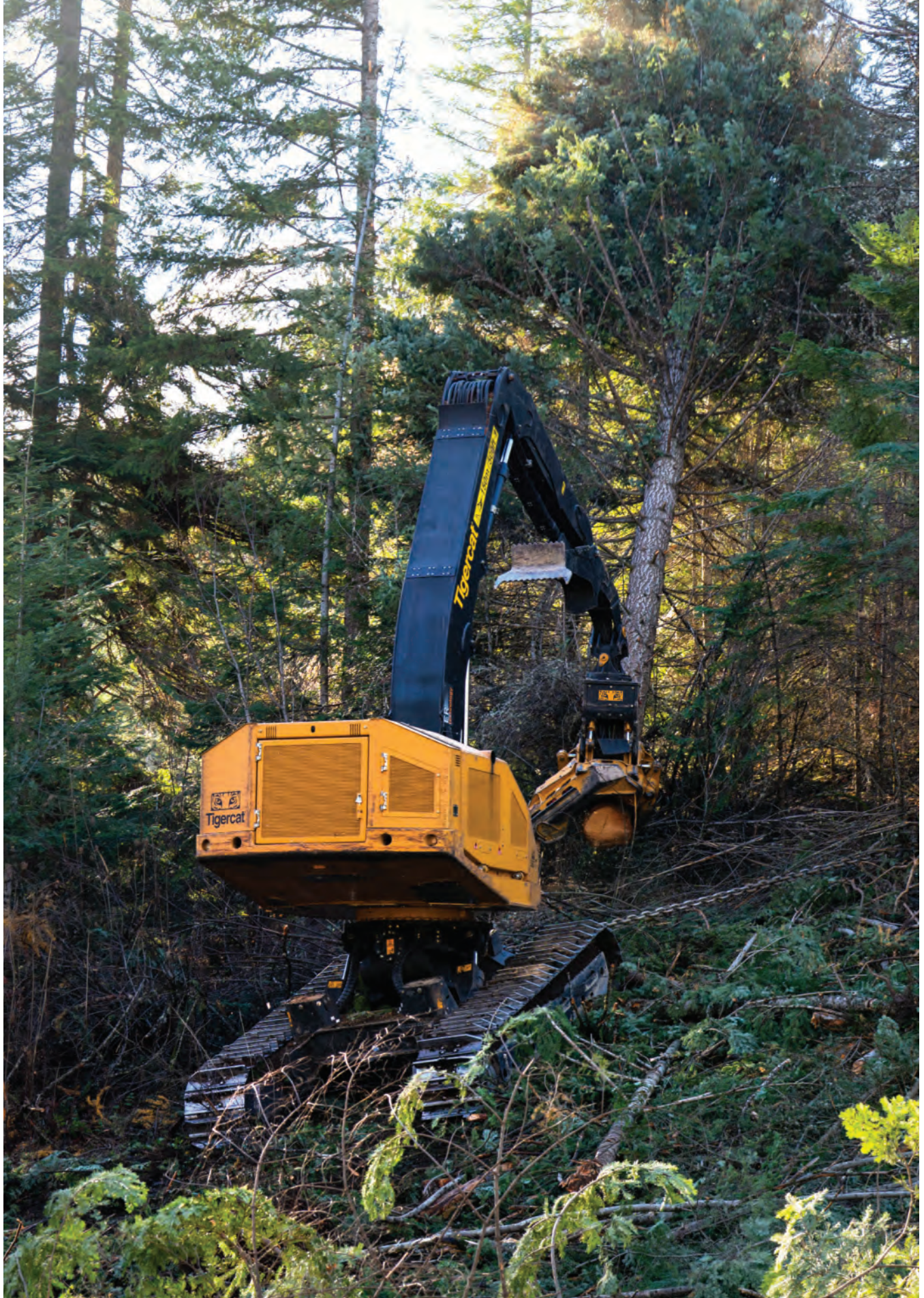
Joe fells and shovels the trees down the slope for Tony to process. Combining felling and shovel logging functions with one machine saves time and money.
