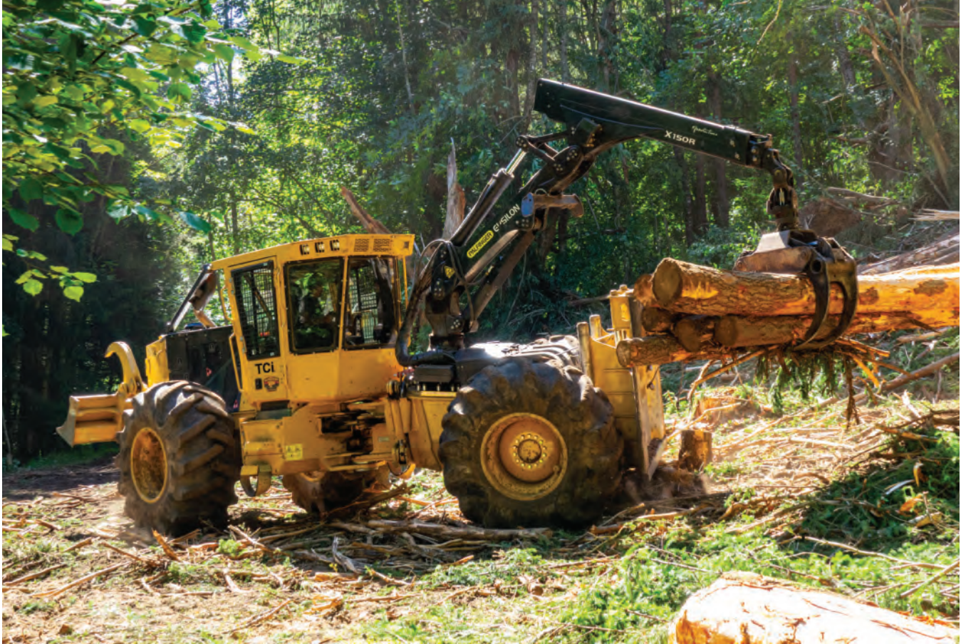
The telescopic crane adds flexibility, allowing the operator to extract trees, build bunches and sort products.
