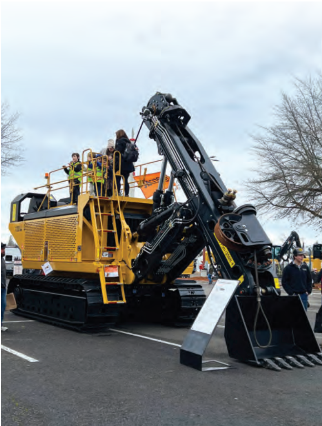
A family on top of the 120 winch assist, a fully remote controlled system engineered for steep slope harvesting.
