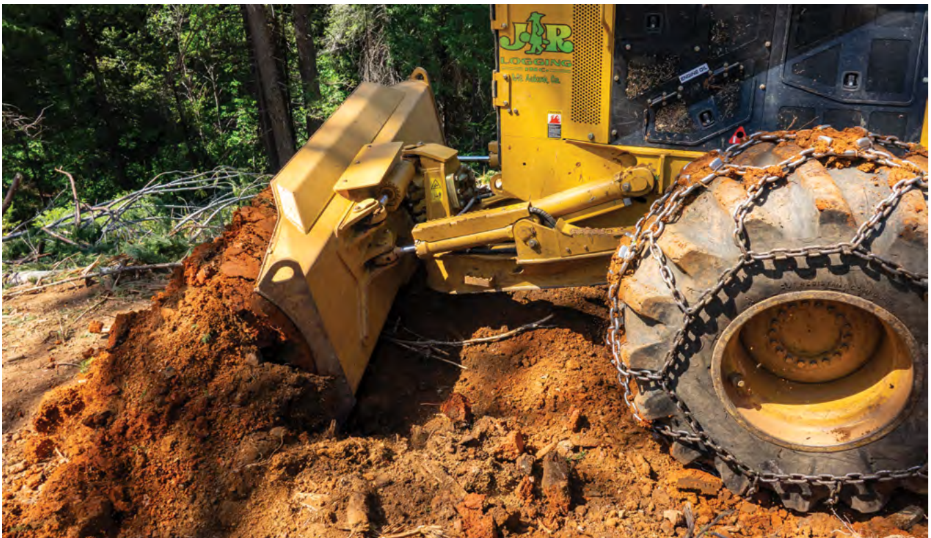
The 620H cuts a water bar to decommission a skidder track. The six-way blade is multifunctional and a great asset on logging operations, allowing the crew to build decks, roads and ditches.
