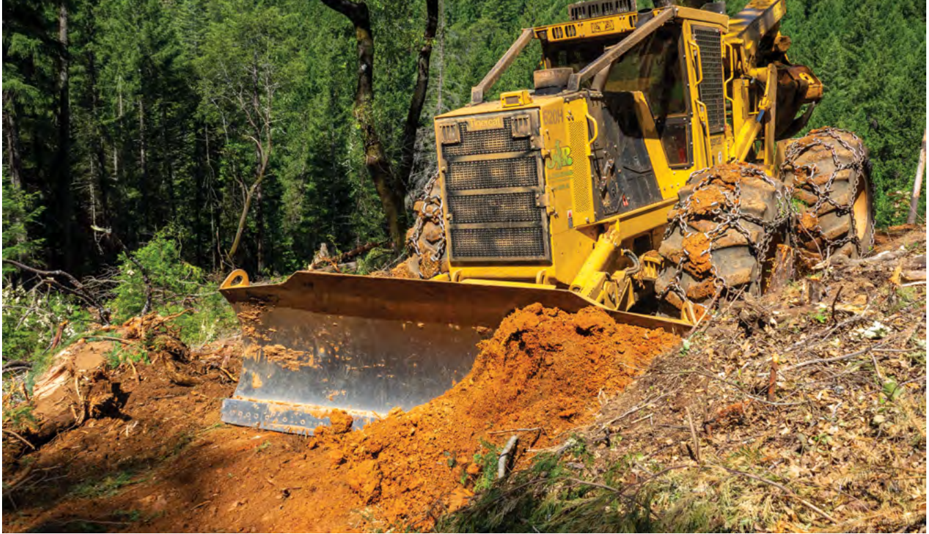
The 620H cuts a water bar to decommission a skidder track. The six-way blade is multifunctional and a great asset on logging operations, allowing the crew to build decks, roads and ditches.
