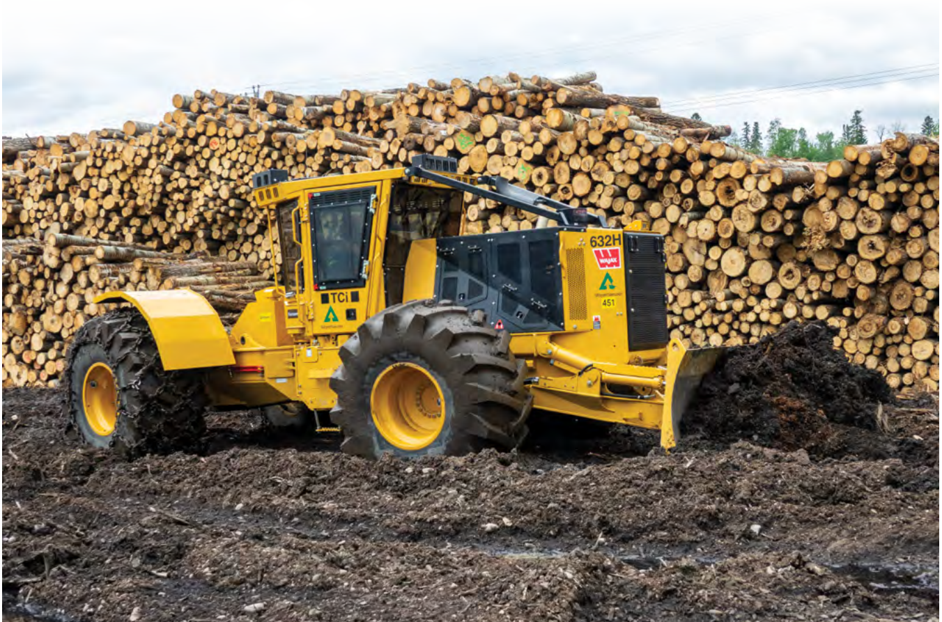
Reclaiming decks in this type of ground condition previously required that the company contract a D6 dozer or excavator. Log Yard Department Lead, Murry Hellekson estimates 80% of the work can now be done with the TCi carrier.
