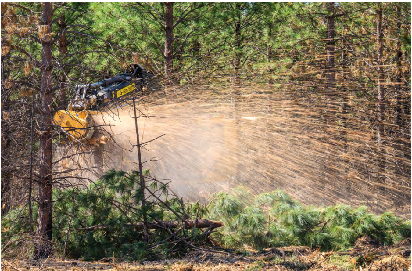
The LX825 hydraulic system is optimized for masticating, delivering high performance, high production rates, and excellent fuel economy. The TCi 4154-15 mulching head is perfectly matched to the carrier.
